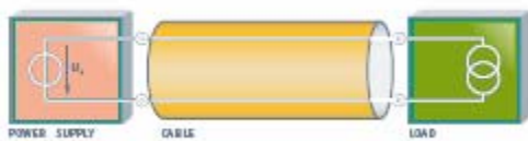
Fig. 5: Simple DART current circuit consisting of a power supply, cable and load.
