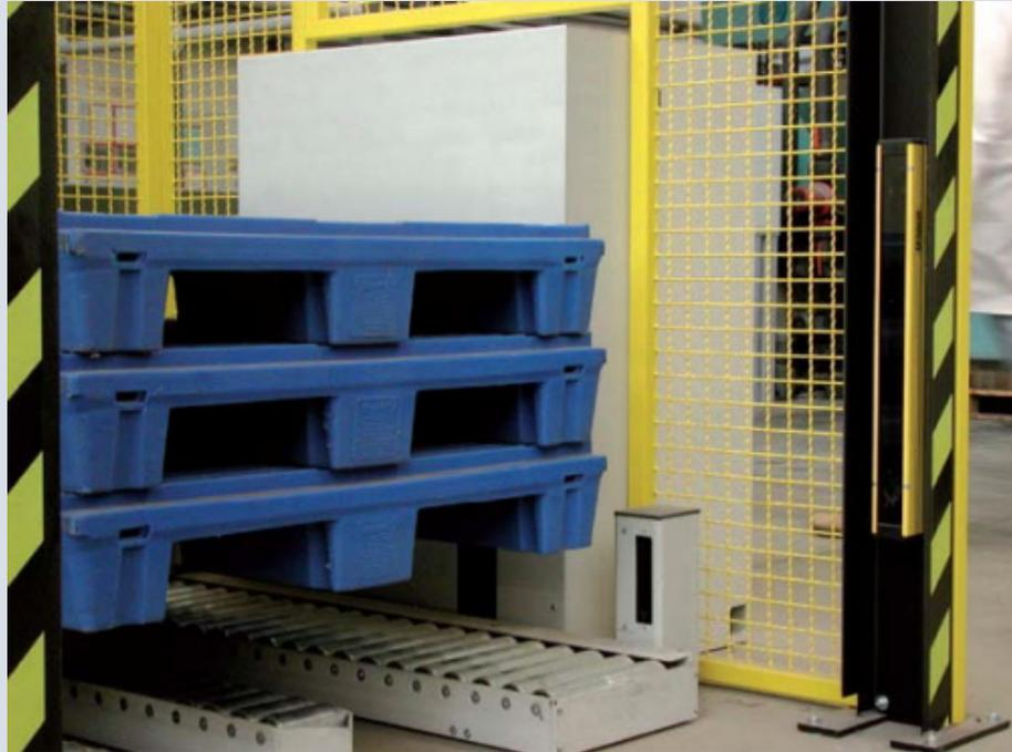
Fig. 3: Pallet accumulator
