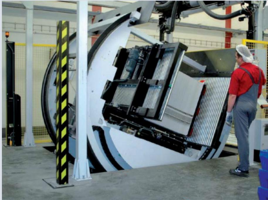
Fig. 1: Stack turner for printed sheets
