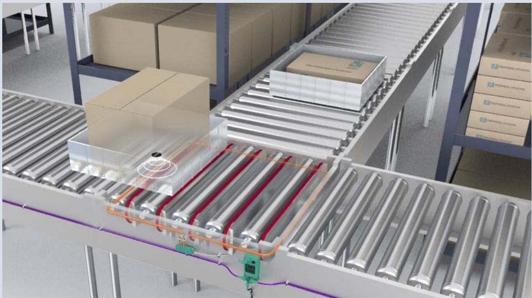
*Conveyor systems based on ethernet solutions that support topology detection can make use of the switch build into the IDENT Control interface to automatically determine the conveyor layout.*
