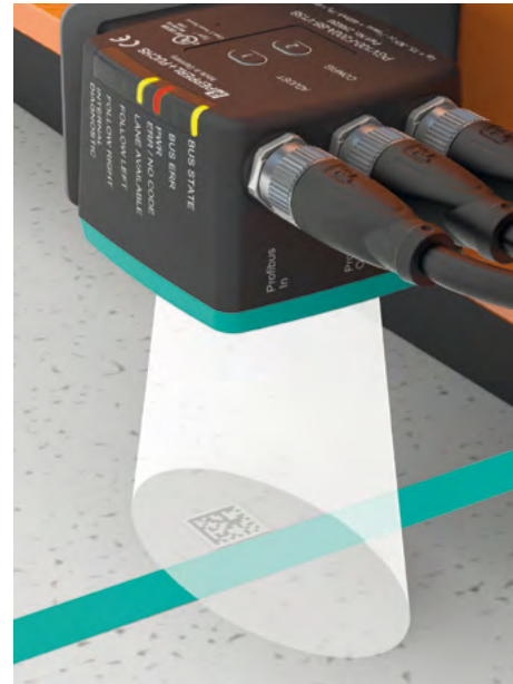
The unique positioning system Position Guided Vision is the first in the world to combine two technologies in one device: optical colored tape/paint tracking for driving and Data Matrix codes for precise position detection of automated guided vehicles.
