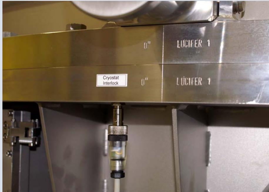
**Fig. 3:** Sensor at the cryostatic temperature regulator
