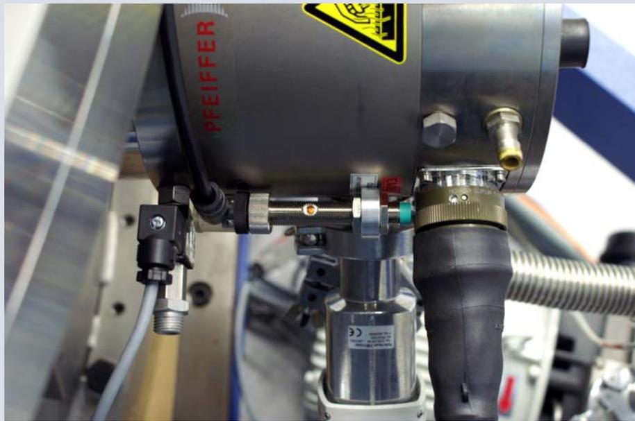
Fig. 2: cable sensor / hose sensor
