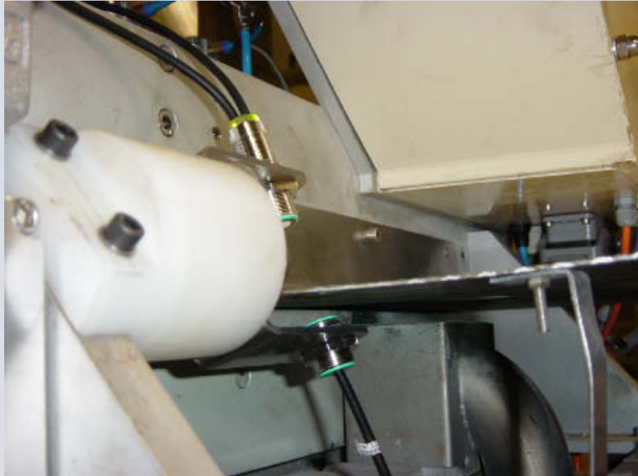
Fig. 2: UGB transmitter below the packaging paper
