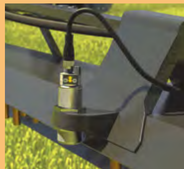
Ultrasonic sensors monitor a constant spray nozzle height above the ground to ensure optimized fertilizer spreading, and prevent damage to the spray arm.
