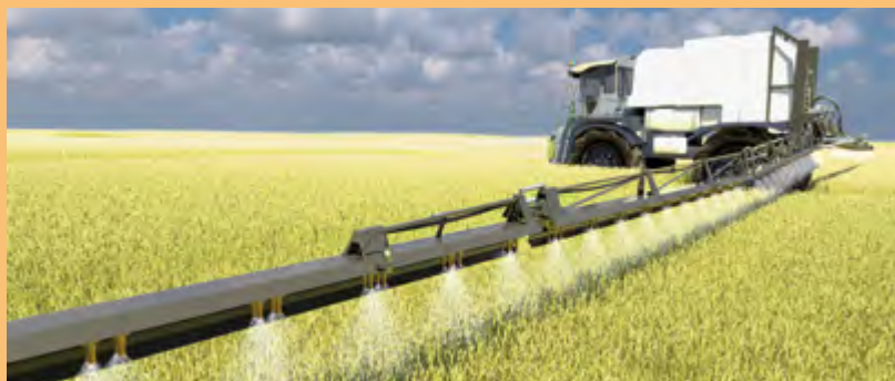
Ultrasonic sensors monitor a constant spray nozzle height above the ground to ensure optimized fertilizer spreading, and prevent damage to the spray arm.
