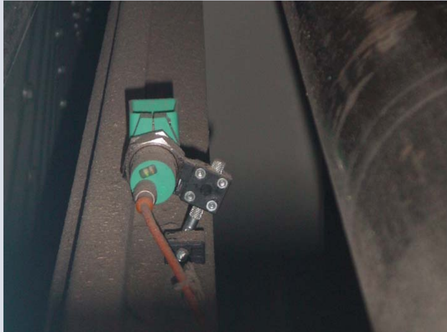
Ultrasonic sensor with attached sound deflector between the roller conveyors
