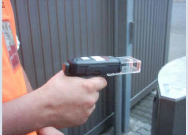
Fig. 3: MAH200 with optical head
