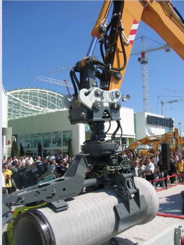
Fig. 4: Quick change system with mounting tool
