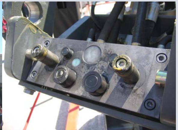
Fig. 3: Mounting tool with fully potted IPC03-16GK data carrier
