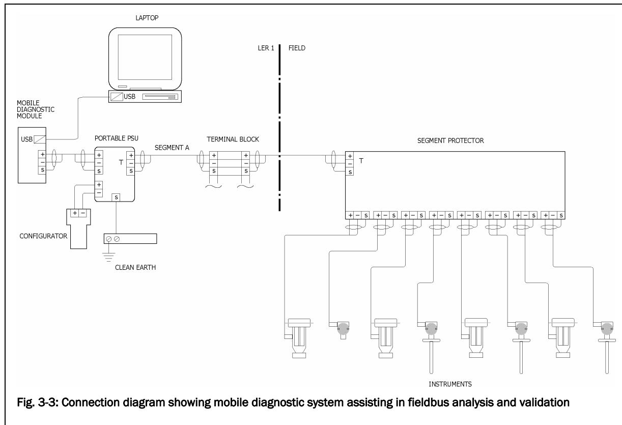
Fig. 3-3: Connection diagram showing mobile diagnostic system assisting in fieldbus analysis and validation
