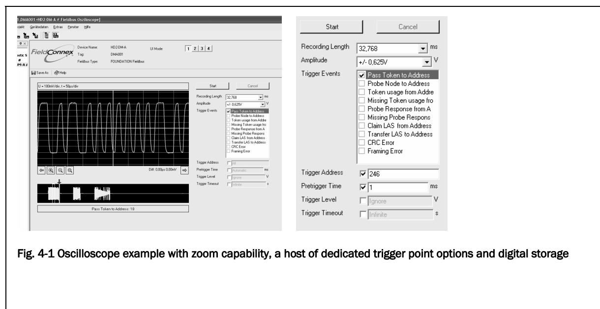
Fig. 4-1 Oscilloscope example with zoom capability, a host of dedicated trigger point options and digital storage
