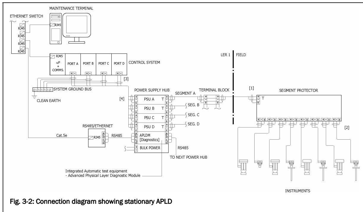
Fig. 3-2: Connection diagram showing stationary APLD
